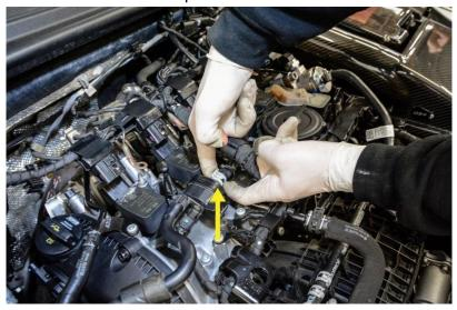
**Step 11**Unclip the coil harness from the plastic clip near oil fill cap.
