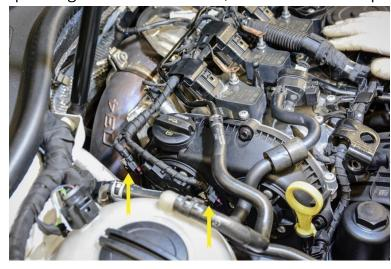
**Step 7**Disconnect the Valve Solenoid Connectors. There should be
