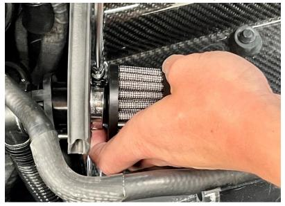
**Step 9** Install the air filter onto the adapter.
