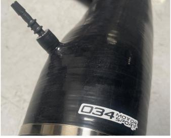
**Step 6** Attach the intake hose to the adapter.
