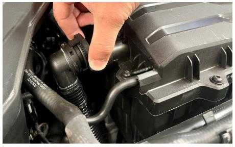
**Step 4** Pull the vacuum line from the airbox.
