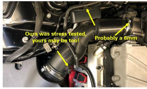
**Step 7**Remove the vacuum line from the intake.
