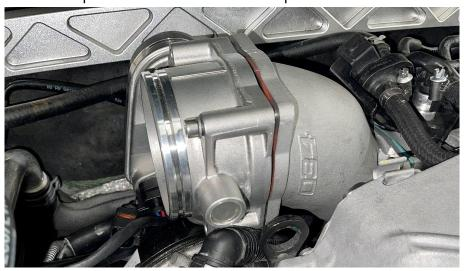
**Step 17**Attach the harness to the new throttle body.
