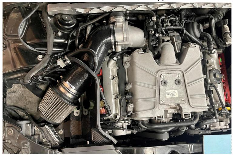
\*If you are planning to use the factory engine cover, the rear piece will need to be notched to fit around the SüperDüper throttle body adapter.\*
