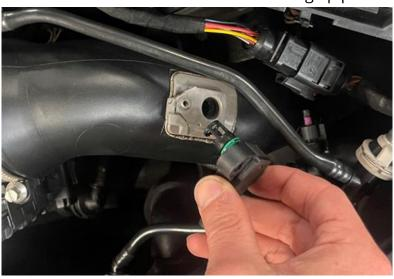
**Step 6**Install the 034 map sensor by pushing it firmly into place.
