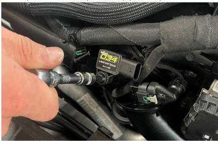
**Step 16** Install the plug-end into the 034 map sensor.
