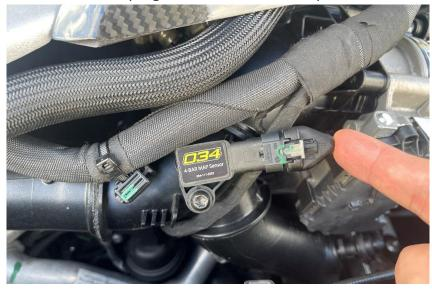
**Step 17**Push the locking clip into the 034 map sensor.
