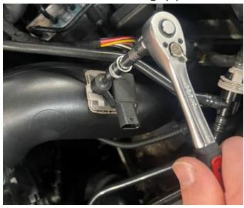
**Step 5**Remove the OE sensor from the charge pipe.
