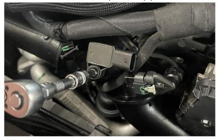
**Step 13**Remove the OE sensor from the pressure pipe.
