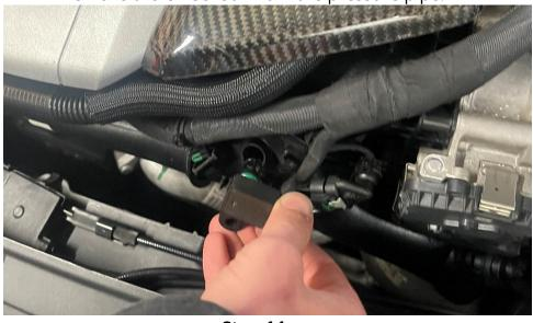
**Step 14** Install the 034 map sensor by pushing it firmly into place.
