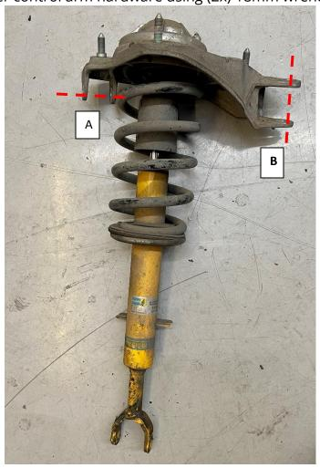
Use the length of the short factory arm as a reference for the 034 short control arm. Install the spherical bearing on the longer arm to its shortest setting. This allows for a factory camber setting.
