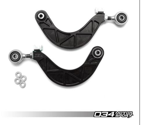
034Motorsport Density Line Rear Adjustable Upper Control Arms are a direct replacement for the stock stamped steel and rubber arms, and allow for approximately 5 degrees of camber adjustment, on top of what the stock eccentric bolt allow.
