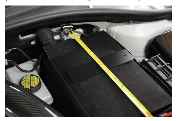
**Step 4** – With the Powdercoated Steel Backing Plate properly located 5.125" from the back of the battery, use a Sharp/Pointy Object to pierce two holes in the factory battery blanket for the Plastic Rivets.
