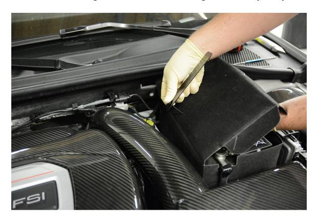
**Step 6** – Install the other Plastic Rivet through the Powdercoated Steel Backing Plate and factory battery blanket as shown below.
