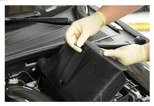
**Step 7** – Secure both Plastic Rivets with the supplied clips as shown below.
