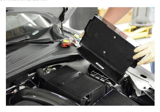
**Step 12 -** Carefully slip the Carbon Fiber Battery Cover into position over the battery blanket.
