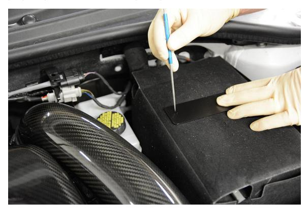
**Step 5** – Install one Plastic Rivet through the Powdercoated Steel Backing Plate and factory battery blanket.
