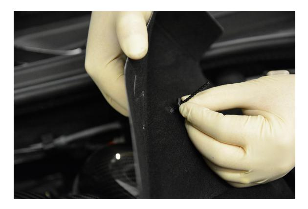
**Step 9** – Trim the ends of the Plastic Rivets using Wire Cutters.
