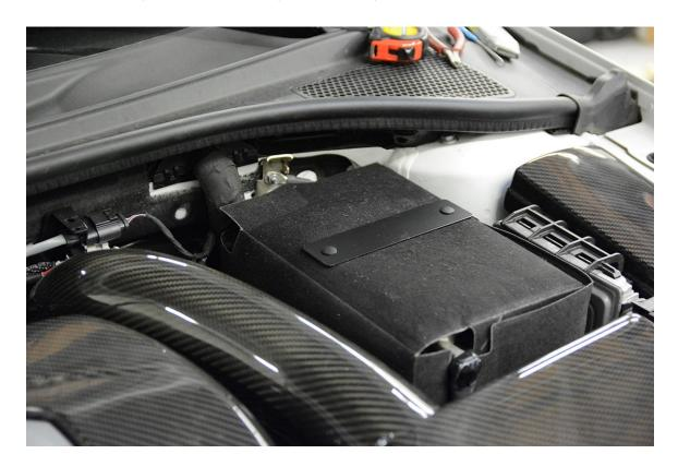
**Step 11** – Properly orient the Carbon Fiber Battery Cover as shown below. **Important:** Ensure that no exposed terminals or wires are in contact with.
