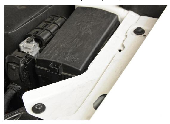
**Step 4** – Using a towel and isopropyl alcohol, thoroughly clean the factory Fuse Box Cover.
