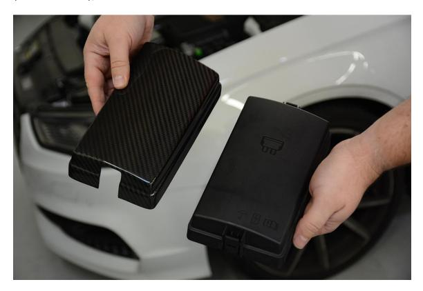
**Step 8** – Slip the Carbon Fiber Fuse Box Cover onto the factory Fuse Box Cover and press firmly to ensure the adhesive strips stick.
