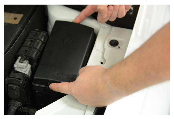
**Step 7** – Make sure that the Carbon Fiber Fuse Box Cover is oriented correctly before attempting installation! It only works if you position it correctly, kind of like rockets and lasers.
