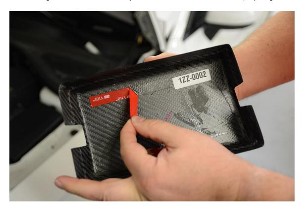
**Step 6** – Remove the factory Fuse Box Cover by pressing in on the tabs at either end, and lifting up.
