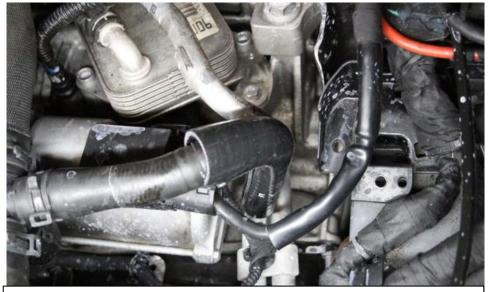
22. Push Hose 1 onto the tube which we rotated the clip on as shown.
