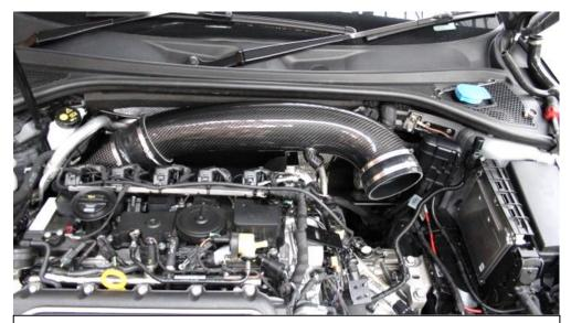
40. Push the carbon tube into the silicon reducer as shown – don't tighten the clamps yet. Optional carbon turbo elbow shown.
