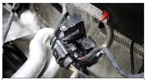
15. Slide the both plugs out of the bracket as shown. Also remove the wire attached to the bottom of the bracket. We will not use the plastic bracket.
