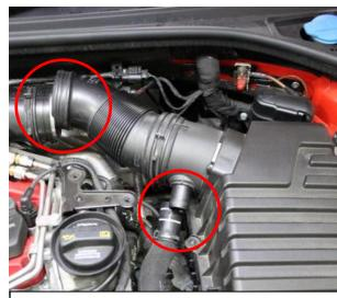
3a. Remove spring clamp from flexi hose at the turbo pipe connection – use an appropriate spring clamp tool. Pull out the flexi hose from the turbo tube. Also remove engine cover and breather hose from the airbox.
