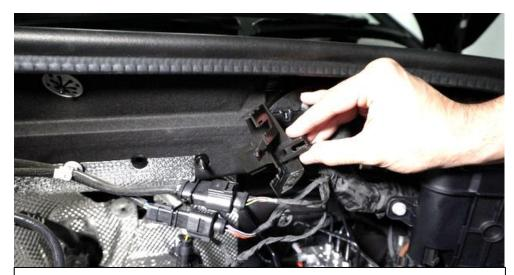
16. Remove the plastic bracket completely.
