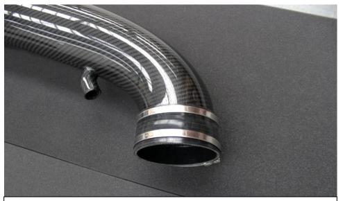
39. Tighten the hose clamp around the carbon tube only. Do not use a ratchet to tighten it - it just needs to be finger tight. Over tightening can damage the tube.
