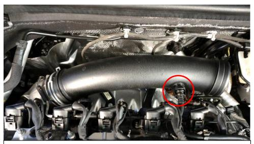
10. Remove the spring clamp holding the turbo tube to the rubber joiner and also the breather connector circled in red.
