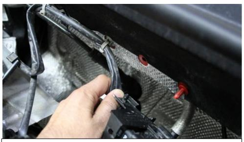
14. We need a bit more slack in the wiring – carefully pull the wiring through the cable ties to allow the plugs to move to the right. You only need a few centimetres extra.
