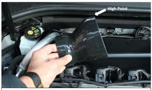
32. Place the reducer onto the stock turbo inlet tube with the appropriate hose clamps and the high point facing upwards as shown.
