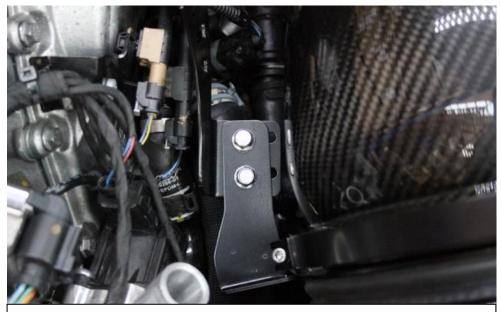
53. Align the holes on the filter bracket with the slots on the engine bracket and push the 2 screws though – it may be easier to push the screws upwards from underneath so that the access is easier for the nuts.
