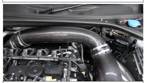
55. Pull the carbon tube into the filter housing, rotate if required for clearance over the brake fluid reservoir and secure the remaining hose clamps. Do not use a ratchet to tighten it – it just needs to be finger tight. Over tightening can damage the tube.
