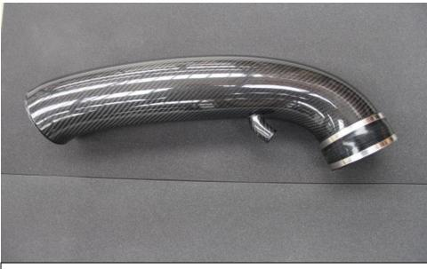
37. Take the carbon tube and place the straight silicon coupler over it with 2 hose clamps.
