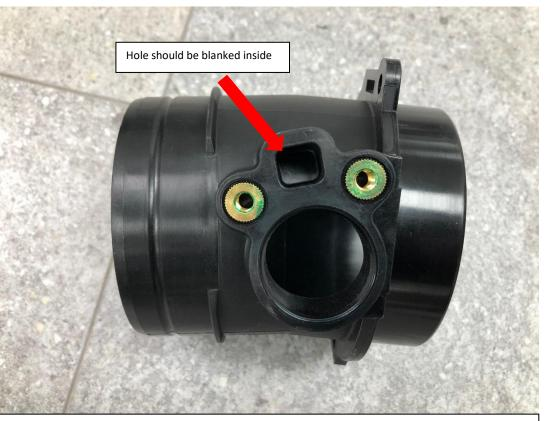
With the breather hose removed you will be able to see this tube connected to the OEM airbox. Please have a look at the square hole as indicated above. This should be blanked off on the inside. So you **SHOULD NOT** be able to see all the way through this square hole. If you can see all the way though this hole and into the tube please **DO NOT** install the intake – contact your Eventuri Dealer.
