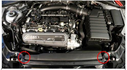
Remove the engine cover. Remove the 2 screws holding the inlet duct in place. Then push the duct into the airbox to release the mounting points and remove duct from engine bay.
