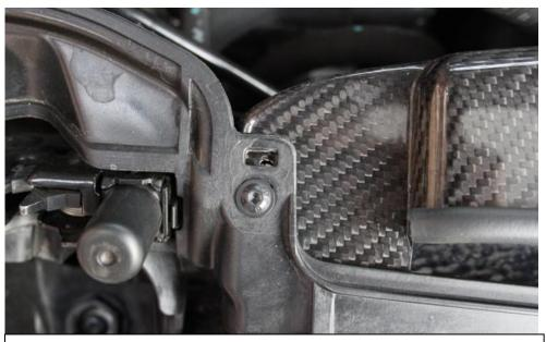
50. – line up the hole on the panel with the correct hole on the duct as shown in previous step. For RS3 Secure with a supplied M5 Screw. For TTRS secure with the original stock screws.
