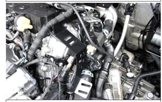
36. Place the new bracket into position as shown on top of the existing bracket. Use the lock nuts to secure – with the triangle locking face should be facing away from the bracket.
