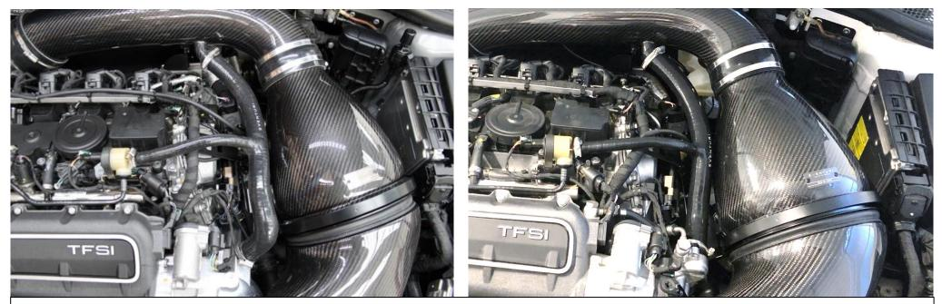
57. Install the breather hose as shown for the 2 variants and secure the hose clamps.
