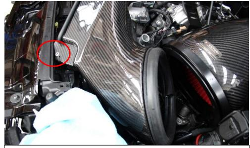
46. Another angle of the duct angled into place – notice the rear edge is inside the slam panel.
