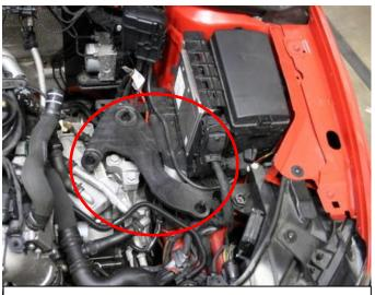
4. Remove entire airbox by pulling upwards. It is held in place with rubber push mounts. Also remove the Airbox mounting tray by unscrewing the 2 bolts.
