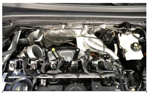
11. Remove the tube from the engine bay.
