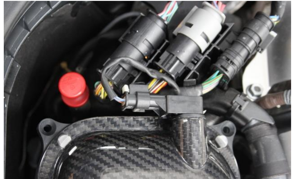
29. Install the MAP sensor plug. Make sure it is fully installed and the locking tab is pushed back in.
