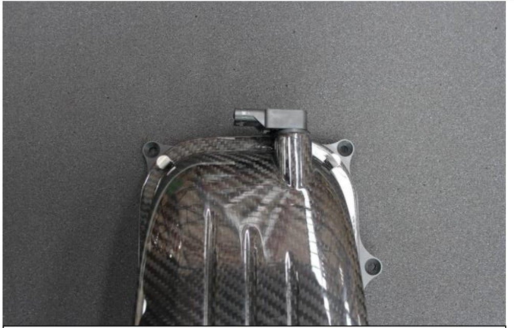
10. Sensor should be rotated 90 degrees to rest on the bracket.
