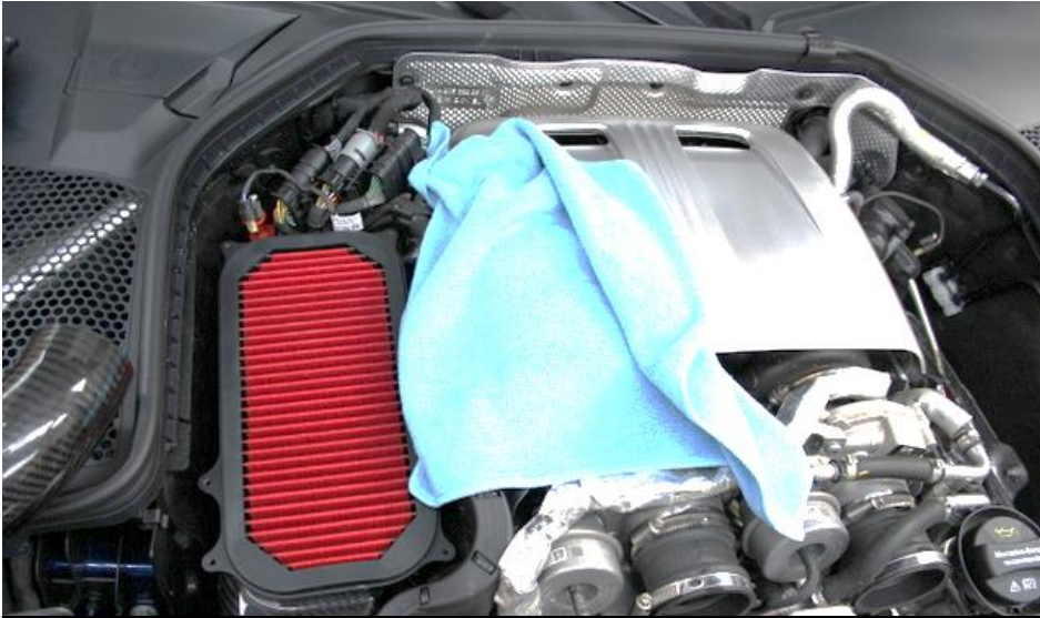
22. Install the filter - make sure it is seated properly all around the flange on the airbox. Place a cloth over the metal engine cover to protect it for the next step.
