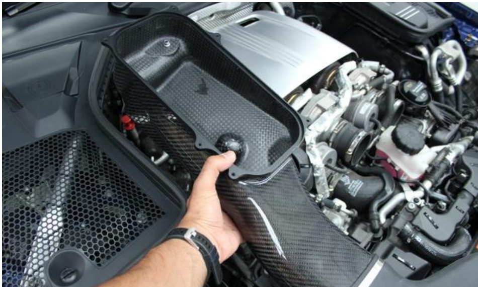
17. Starting with the left side we will install the base first. Before installing please see next step. The rubber mount at the back of the airbox needs to be lined up.
