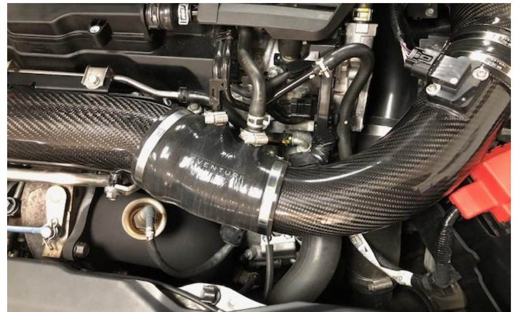
36. Ensure the carbon MAF tube is pushed into the silicon. Secure all hose clamps.
