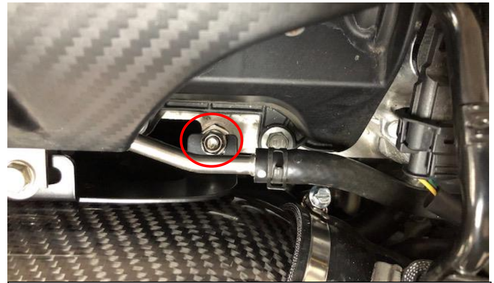
32. Secure the tube with the supplied M6 Flanged nut over the anti-vibration Mount.
