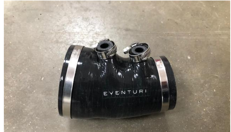
34. Take the new Silicon hose and use the 2 small hose clamps from your previous silicon hose removed from the intake (removed in step 2).
