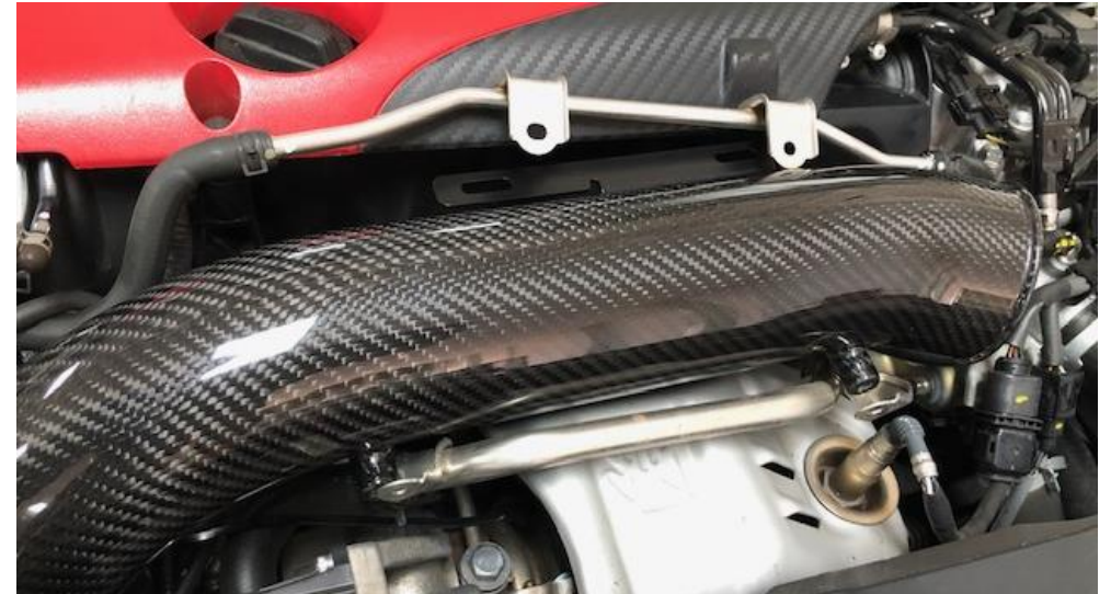
26. Carefully lower the tube into place.
