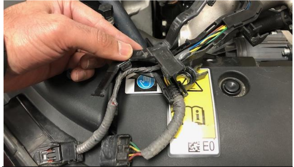
10. Using a flat head screwdriver – carefully start to prise open the clips around the plastic cover. Start from the top and work your way down opening the cover as you go.
