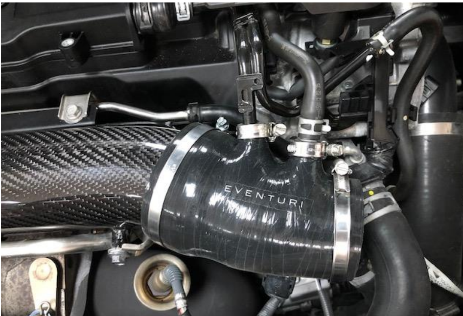
35. Install the new silicon hose.
