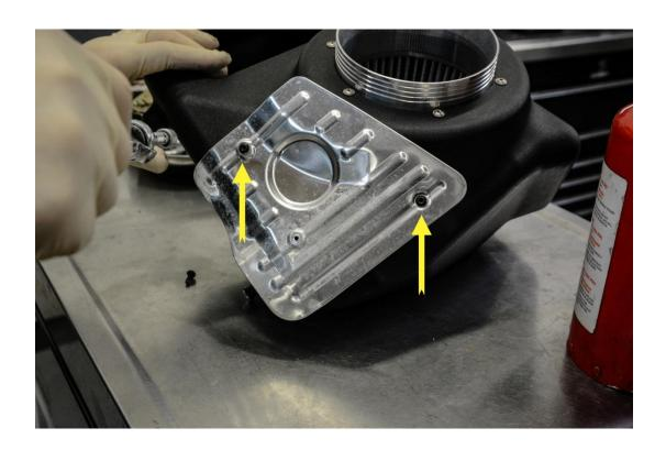
**Step 11** – Install the 3 factory rubber grommets on the bottom of the P34 Cold Air Intake air box.
