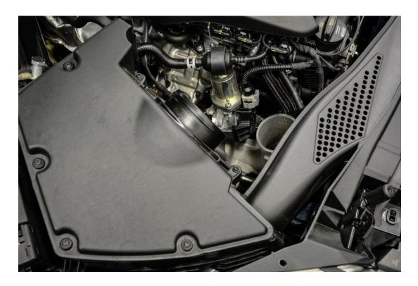
**Step 6** – Lift up the factory air box to pop it free from the mounting grommets, then rotate as needed to get around the factory inlet duct.
