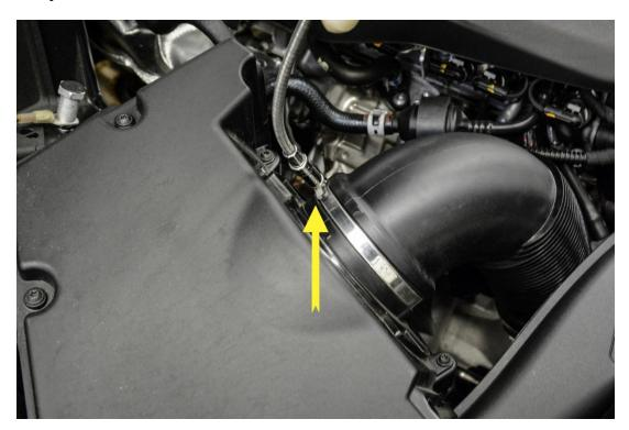
**Step 4** – Once both hose clamps have been loosened, remove the vacuum hose from the intake tube.
