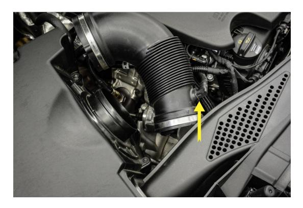
**Step 5** – With the vacuum hose disconnected from the intake hose, remove the factory intake hose from the car. Your engine bay should look as the photo below.
