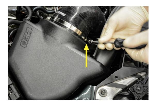
**Step 17** – Once the hose clamps are secure and the inlet hose is snug to the turbo inlet and air box, reconnect the vacuum line to the inlet hose.
