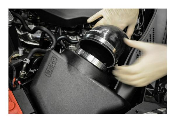
**Step 15 –** Using an 8mm Hose Clamp Driver or Socket, tighten the lower hose clamp first, securing the inlet hose to the turbo inlet.
