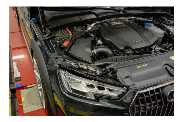
**Step 2** – Using an 7mm Hose Clamp Driver or Socket, loosen the hose clamp securing the intake tube to the turbo inlet.
