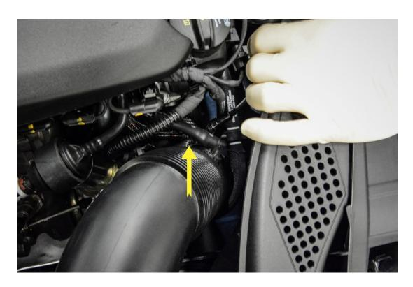
**Step 3** – Using a 7mm Hose Clamp Driver or Socket, loosen the upper hose clamp, securing the intake tube to the factory airbox.
