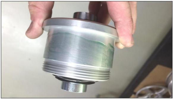
4. See figure below. Slide the carrier into the bore in the arm with a slight turning motion to further spread the Loctite around. It does not matter from which side of the arm you install the carrier, but it is preferred if both sides of the car were the same. The carrier should sit flush against the surface of the control arm.
