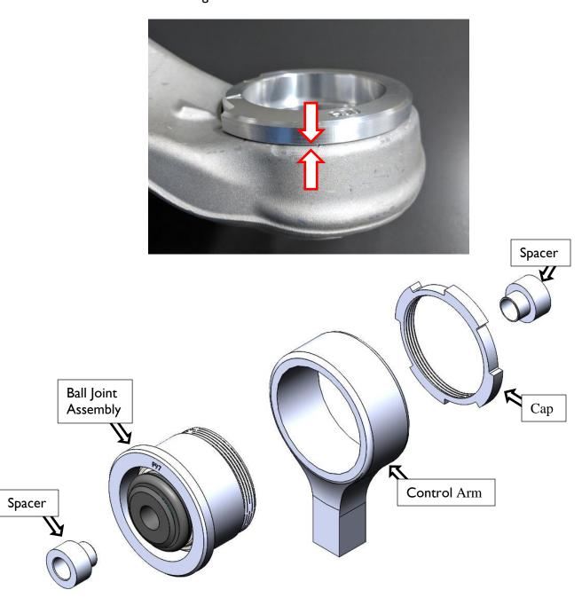
5. Install the Dinan retaining cap onto the arm. Put a small amount of Loctite on the internal threads of the cap and torque to 110 foot-pounds to secure the retaining cap. A special Dinan cap tool is included in every kit. This tool is used with a 1/2" torque drive. Set torque wrench to 110 foot-pounds and do not concern yourself with a conversion factor. See figure below.
