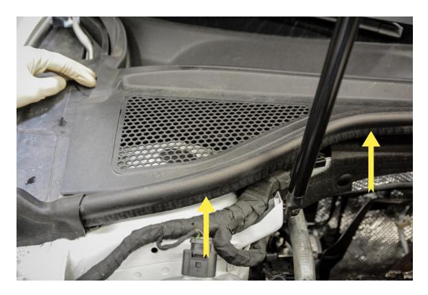
**Step 3** – With the weather stripping removed and the plastic cowl cover lifted, locate the bolt securing the dust shield to the strut tower.
