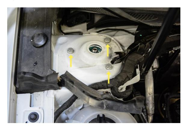
**Step 21 -** Reinstall dust shield and factory bolt using 10mm Socket. Place weather stripping back on cowl cover.
