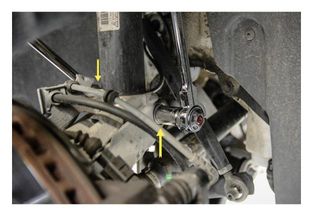
**Step 10A** – Once lower strut bolt and nut are removed, use a Spreader Socket to separate the strut housing from the lower knuckle. Spreader Socket pictured below.
