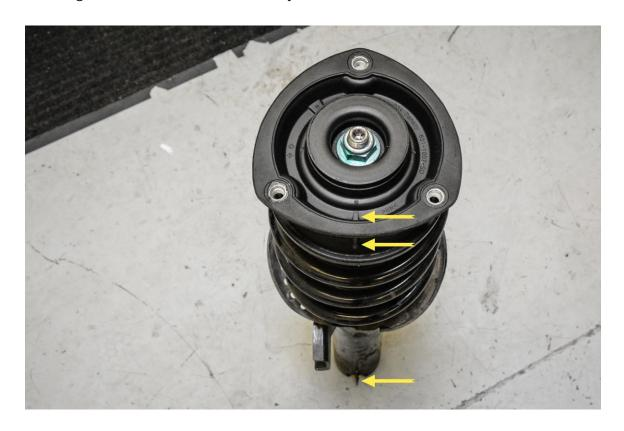
**Step 16 -** Once upper strut nut is torqued, remove spring compressors and marvel at your work. You're ready to reinstall!
