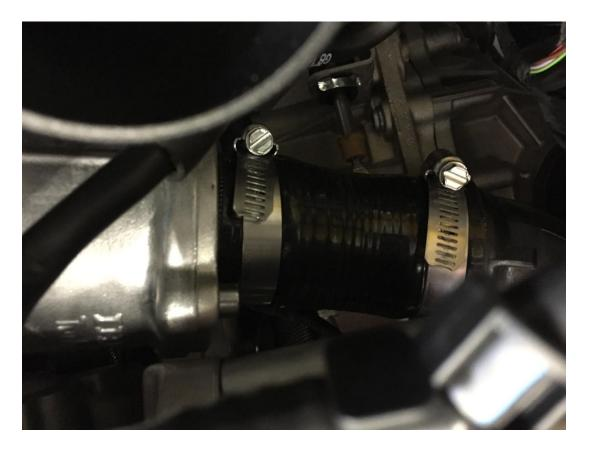
**Step 10** – Loosen the throttle body hose clamps shown below. The hose will be removed from underneath the vehicle.
