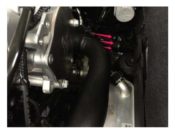
**Step 9** – Pre-install supplied clamps onto the Silicone Turbo Outlet Hose. Slide into place at the turbo and push the charge pipe back onto the hose. Tighten clamps.
