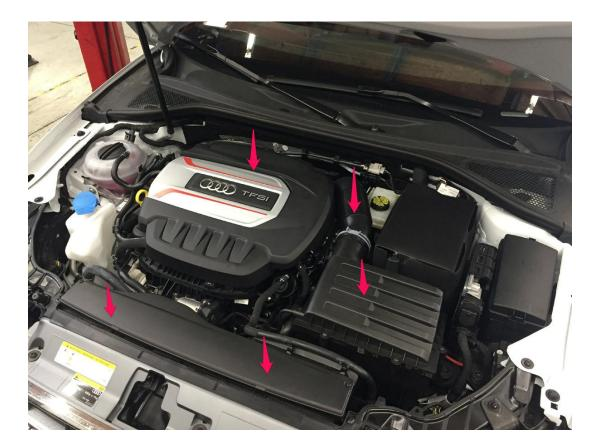
**Step 2** – To remove the air inlet duct, unclip hoses and unscrew the T2 Torx screws shown below.
