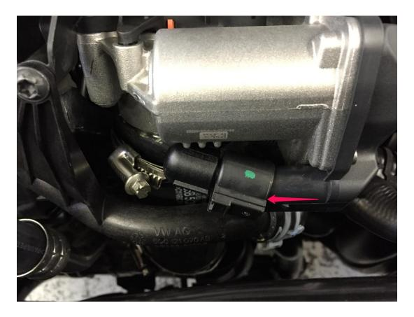
**Step 18 (Optional)** – Remove the mounting screws for the coolant tube pictured below.
