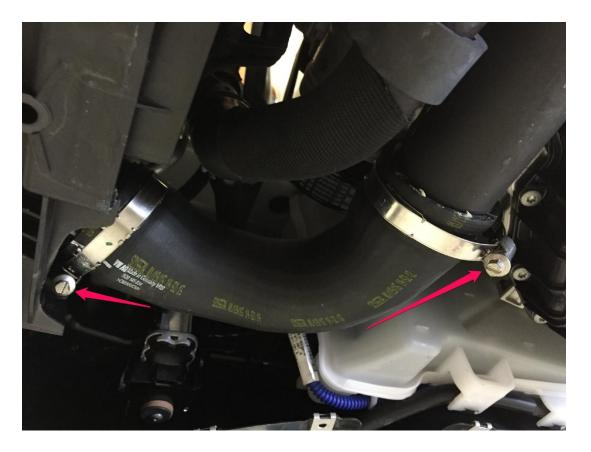
**Step 15** – Now you will continue removal of the throttle body hose, which was started in Step 10. First, loosen the charge pipe mounting bolts, located near the arrows below.
