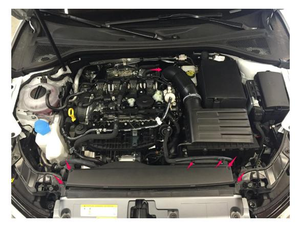
**Step 3** – You will also need to unclip the second half of the air scoop at the airbox after removing the lid, then slide out the whole piece to make room.
