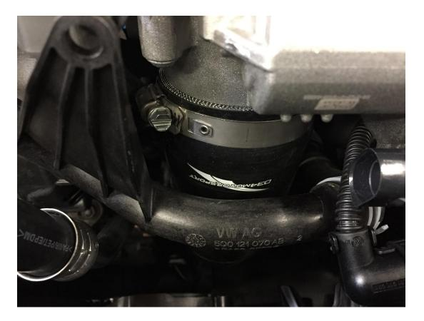
Step 20 – Reinstall the charge pipe, coolant tube, and connectors in reverse order. You're done!
