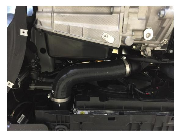
**Step 14** – Locate the intercooler outlet hose on the passenger side of the car. Remove it after loosening the factory clamps with a hose clam driver. Install the 034Motorsport Silicone Intercooler Outlet Hose using the supplied clamps.
