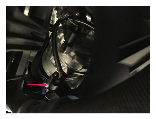
**Step 17** – Disconnect the Throttle Body Connector (shown below) from the Throttle Body. This will provide more space to access the Throttle Body Hose.
