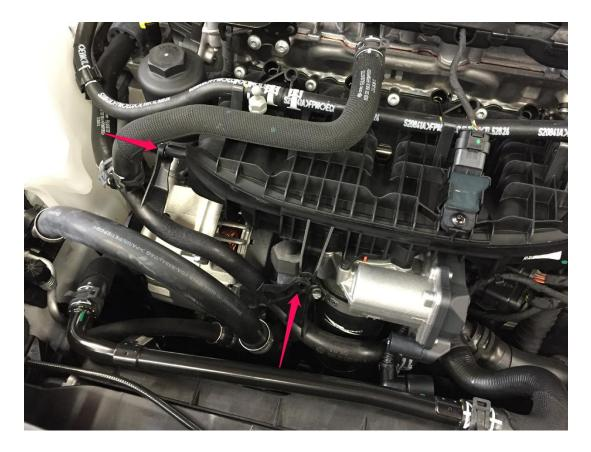
**Step 19** – With a loosened charge pipe, loosened clamps, and disconnected MAP Sensor, remove the factory throttle body hose. Pre-install clamps on to 034Motorsport Silicone Throttle Body Hose and be sure to orient clamps for easy access when tightening. Install the new hose and clamps onto the throttle body.
