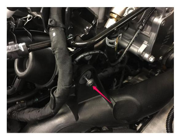
**Step 6** – Locate the turbo outlet hose and loosen the clamps shown below.
