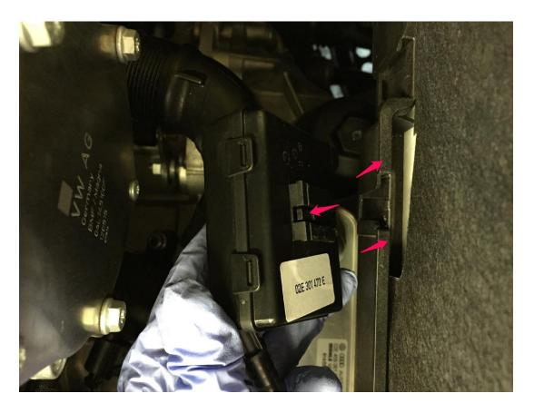
**Step 8** – Pull the charge pipe toward the battery to remove the hose.
